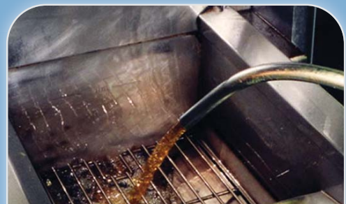
CLEAN FRYER OUT. RETURN THE FILTERED OIL TO THE VAT
