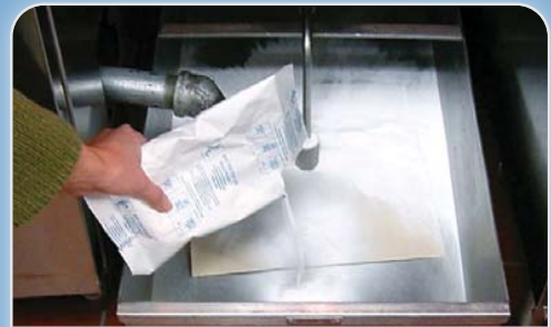
SPRINKLE MAGNESOL OVER FILTER PAPER
