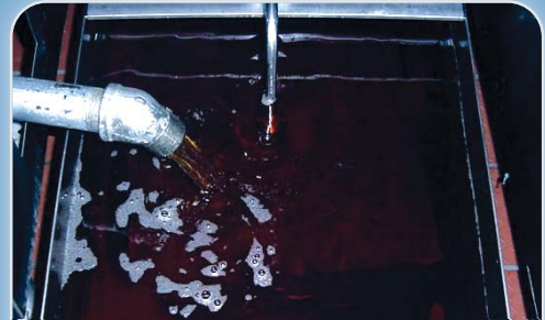
DRAIN THE OIL FROM FRYER INTO THE FILTER PAN
